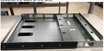
Note The outer rail can be removed from the ThunderRack chassis to allow for ease in mounting the rails to the rack
