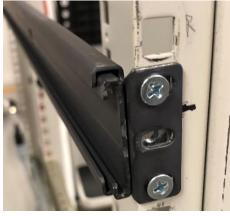
5. Insert ThunderRack into mounted rack rails
