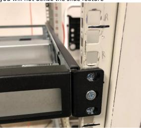
8. ThunderLink Adapters may be added at the beginning or swapped out once racked by removing the brace from the middle of rack
